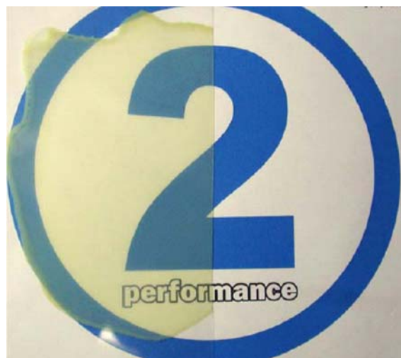
Fig. 2 High transparent-conductive ITO/PVP nanocomposite film
